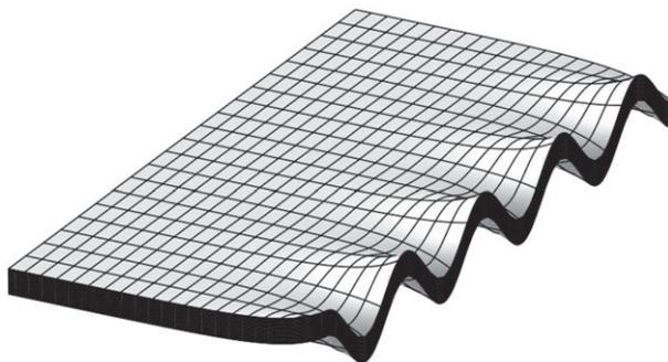
**Figure 2.** Buckling wrinkles with wavenumber  $k$  localized near the edge of a compressed thin plate with thickness  $h$ .
