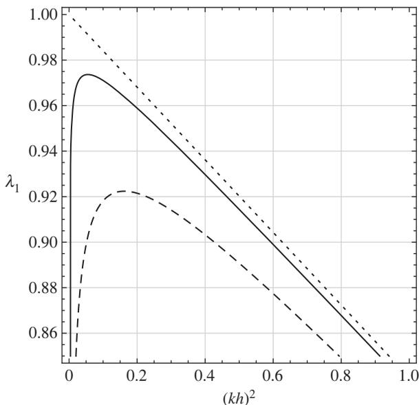
**Figure 4.** Bifurcation curves for the appearance of edge wrinkles on a thin plate resting on a local foundation whose elastic modulus  $\kappa = (h/\ell_s)^4 \mu k$  is proportional to the wavenumber  $k$ . The curves are for uni-axial pre-stress and foundation relative compliance  $h/\ell_s = 0$  (dotted),  $1/3$  (solid) and  $1/2$  (dashed).
