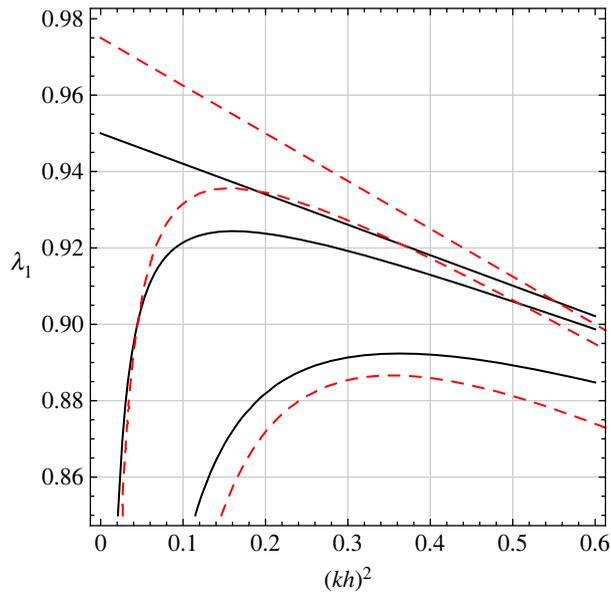
**Figure 5.** Edge (solid) versus body (dashed) bifurcation curves for a thin incompressible elastic plate resting on a Winkler foundation with relative compliance  $h/\ell_s = 0, 1/3, 1/2$  in a state of bi-axial pre-stretch ( $\lambda_1 < 1, \lambda_2 = 1.05$ ). Body wrinkling takes place in compression and parallel to the edge (i.e.  $n_2 = 0$ ); it occurs prior to edge wrinkling for  $h/\ell_s = 0$  and  $1/3$  and after it for  $h/\ell_s = 1/2$ . (Online version in colour.)
