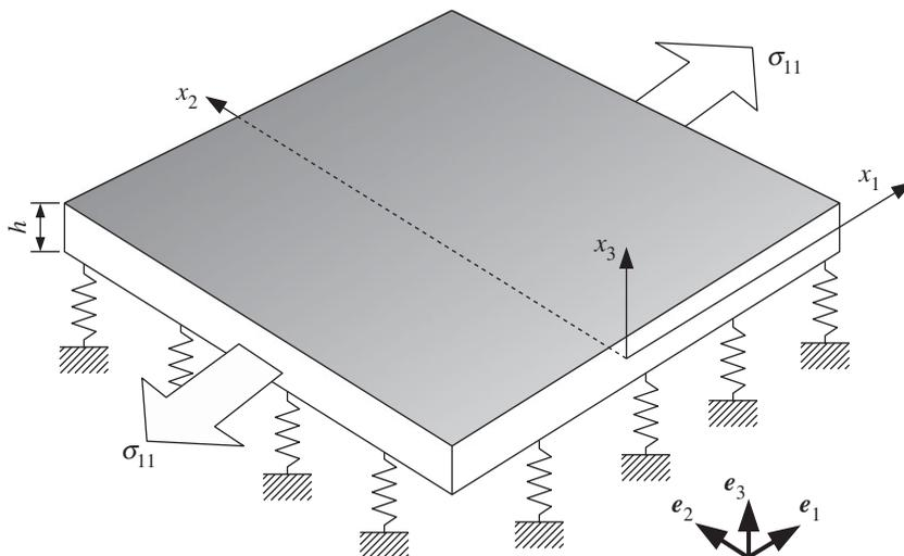
**Figure 1.** Hyperelastic semi-infinite plate resting on a Winkler foundation. Here the plate has been homogeneously pre-stretched along  $x_1$  (equilibrium configuration) by the application of a uni-axial stress  $\sigma_{11}$ .
