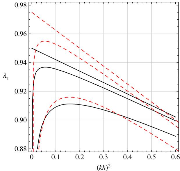
**Figure 6.** Edge (solid) versus body (dashed) bifurcation curves for a thin incompressible elastic plate resting on a local foundation with stiffness  $\kappa = (h/\ell_s)^4 \mu k$  proportional to the wavenumber  $k$  and relative compliance  $h/\ell_s = 0, 1/3, 1/2$ , in a state of bi-axial pre-stretch ( $\lambda_1 < 1, \lambda_2 = 1.05$ ). Body wrinkling takes place in compression and always prior to edge wrinkling. (Online version in colour.)
