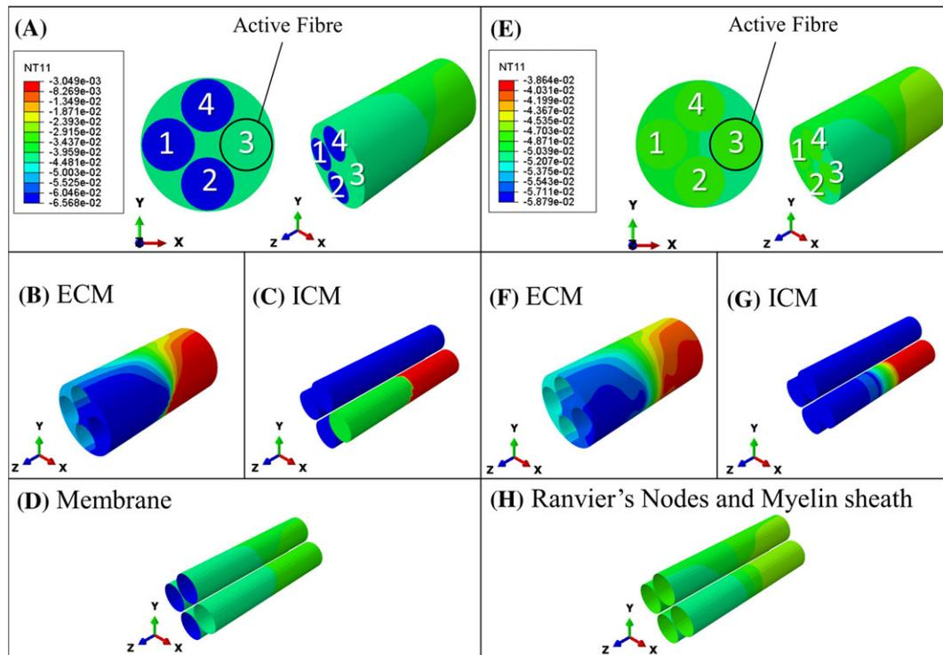
**FIGURE 9** Voltage distribution (NT11) in an unmyelinated nerve bundle, in (A) to (D), and in a myelinated nerve bundle, in (E) to (H), for 5% elongation. Frontal and isometric view of an unmyelinated and myelinated nerve bundle model in (A) and (B), respectively. In (B) and (F), the ECM, in (C) and (G) the ICM of the 2 bundle types. In (D), the isometric view of the nerve membrane and, in (H), the Ranvier's nodes and the myelin sheath of the myelinated bundle
