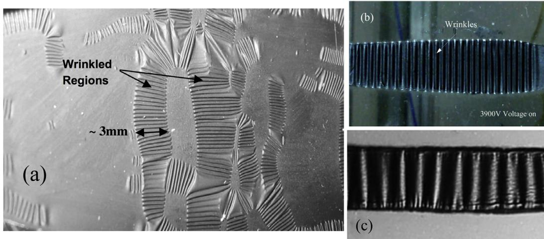
**Fig. 2.** Experimental evidence of electro-mechanical wrinkling instability: (a) collapse of a thin film of the rubber-like material VHB 4905/4910 put under a large voltage (Plante and Dubowsky, 2006); (b) wrinkling of a VHB 4910 membrane under high voltage (Liu et al., 2016); (c) electric activation of acrylic elastomers (Pelrine et al., 2000). We estimate that the ratio of the initial plate thickness to the wrinkle wavelength is  $H/L \simeq 0.17, 0.35$  in Cases (a) and (b), respectively.
