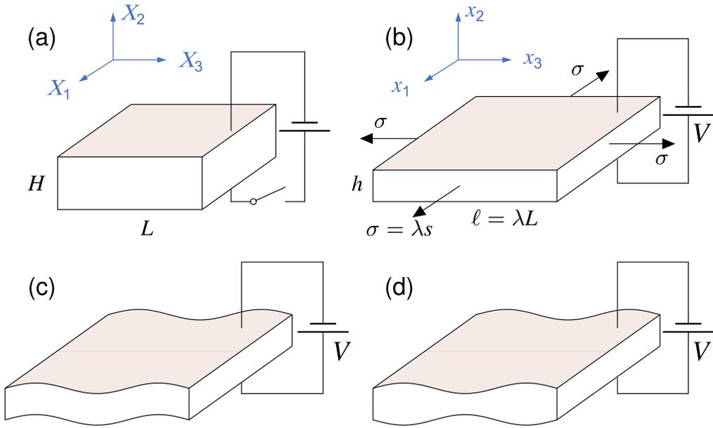
Fig. 3. When put under voltage  $V$  and/or stress  $\sigma$ , a rectangular plate made of a soft dielectric and with faces covered by compliant electrodes deforms homogeneously (a) and (b). It can even deform so severely as to lose its stability and buckle into antisymmetric (c) or symmetric (d) modes of wrinkles.
