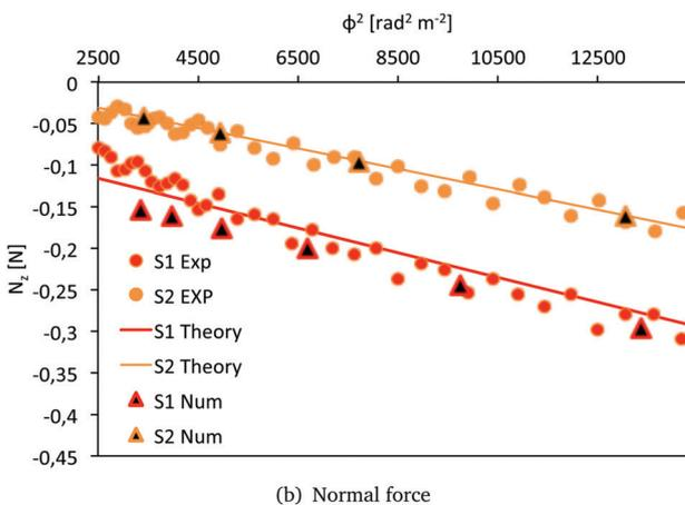
**Fig. 5** Comparison of the resultant torque  $\tau$  and normal force  $N_z$  for S<sub>1</sub> and S<sub>2</sub>. Results of the numerical simulations in Abaqus (triangles), analytical predictions with the models (8) and (9) (solid lines) and experimental data (red circles for S<sub>1</sub> and orange circles for S<sub>2</sub>).
