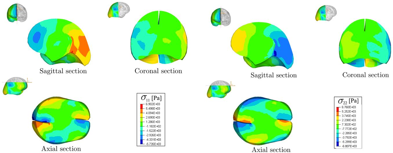
Figure 4: Results of the FE simulations of a rotational head impact, performed with the UCDBT Model. Distribution of the principal Cauchy stress components  $\sigma_{11}$  (on the left) and  $\sigma_{22}$  (on the right) in the Sagittal, Coronal and Axial planes. Here the orange and blue areas correspond to peak stress magnitude of approximately 4 kPa, same as for the vertical stress component  $\sigma_{33}$ , see Figure 6 in the main paper.
