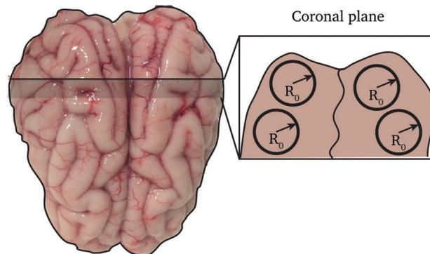
Fig. 2 Sketch of the cutting map of a fresh porcine brain (top view). The cylindrical samples were obtained by cutting a slice of brain excised from the coronal plane into cylinders of radius  $R_0 = 10 \text{ mm}$ .
