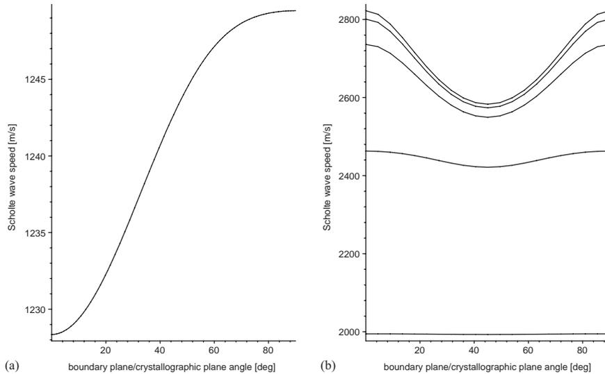
Fig. 2. Scholte wave speeds for (a) Water/Terpine interface and (b) Methanol/Germanium interface, where the speed of sound in the fluid is (m/s): 2000 (bottom curve), 2500, 3000, 3500 and 4000 (top curve).
