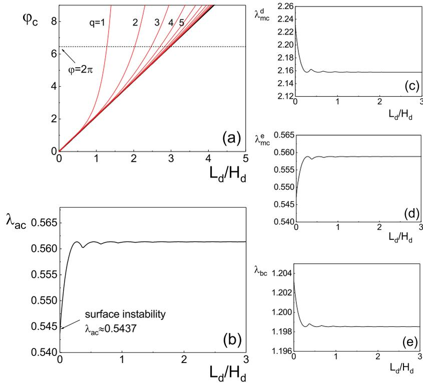
**Fig. 7.** Bending instability of a neo-Hookean ( $C^d = C^e = 10^4$ ) dielectric-elastomeric bilayer with  $\bar{H} = \bar{\mu} = 1$ : the critical bending angle  $\varphi_c$  and the critical stretches  $\lambda_{ac}$ ,  $\lambda_{mc}^d$ ,  $\lambda_{mc}^e$  and  $\lambda_{bc}$  at the onset of buckling versus the width aspect ratio of the dielectric elastomer  $L^d/H^d$  are shown in (a)–(e), respectively.
