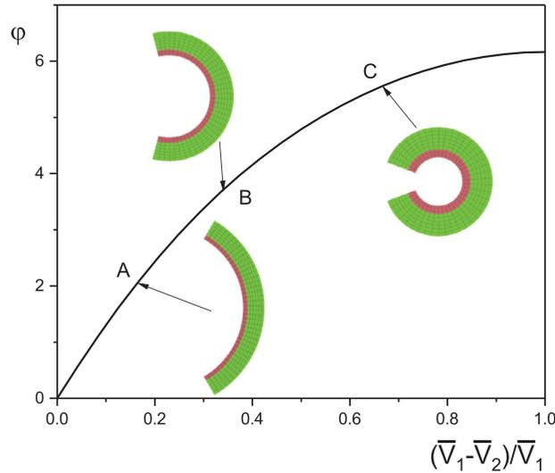
**Fig. 5.** Plot of bending angle  $\varphi$  as the function of voltage change  $(\bar{V}_1 - \bar{V}_2)/\bar{V}_1$  for a dielectric-elastic bilayer with  $L^d/H^d = 3$ ,  $H^e/H^d = 1$ ,  $\mu^e/\mu^d = 10$  and  $G^d = G^e = 46.3$ . The applied voltage to stretch the dielectric block is  $\bar{V}_1 = 1.2$  and then is reduced gradually to zero. For the bilayers A, B and C, we have  $\bar{V}_2 = 1, 0.8$  and  $0.4$ , respectively.
