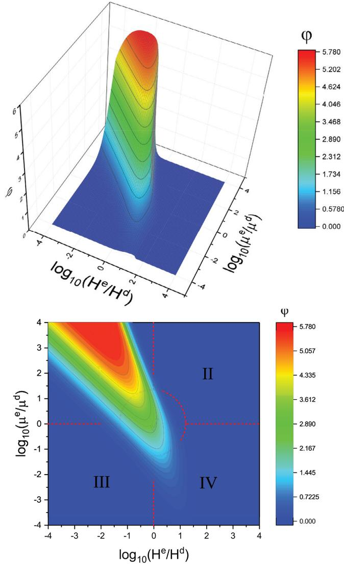
**Fig. 6.** Plot of bending angle  $\varphi$  as a function of  $\log_{10}(H^e/H^d)$  and  $\log_{10}(\mu^e/\mu^d)$  for a dielectric-elastic bilayer in the case where  $L^d/H^d = 3$  and  $G^d = G^m = 46.3$  (top) and its top view version (bottom). The applied voltage to initially stretch the dielectric block is  $\bar{V}_1 = 0.8$  and then it is completely released ( $\bar{V}_2 = 0$ ).
