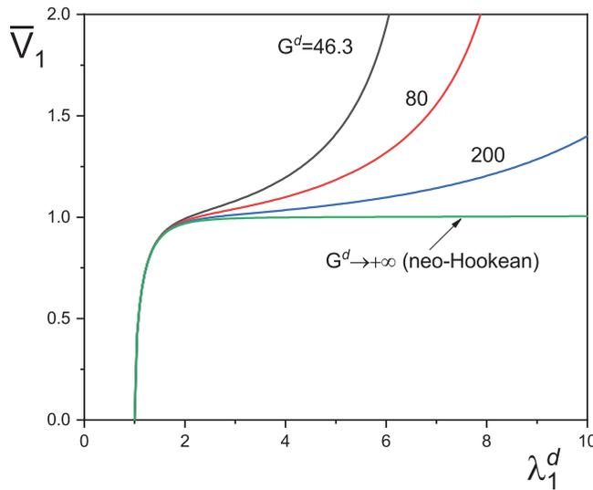
Fig. 3. Nonlinear behaviors of Gent dielectric elastomers for varying  $G^d$  subject to a voltage  $\bar{V}_1$ . The Gent model degenerates to the neo-Hookean model in the limiting case  $G^d \rightarrow \infty$ .
