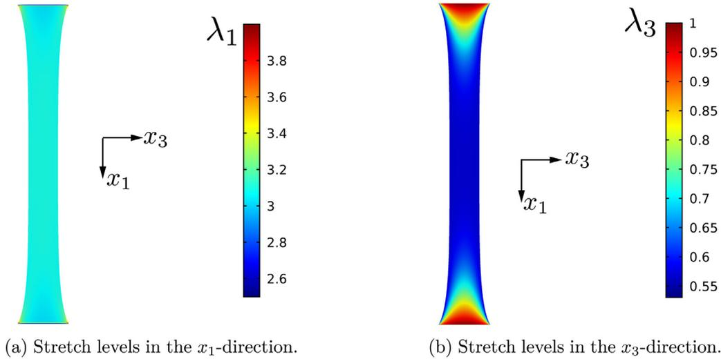
**Fig. 6.** Stretches in the dielectric plate after uni-axial loading by a weight, prior to activation, as computed by FE analysis using COMSOL Multiphysics®. We used the same physical characteristics as those in the experiments by [Keplinger et al. \(2010\)](#). Dimensions: length 100 mm; width 50 mm; thickness 1 mm. Attached mass: 150 g. Constitutive model: neo-Hookean dielectric with  $\mu = 9833.07$  Pa.
