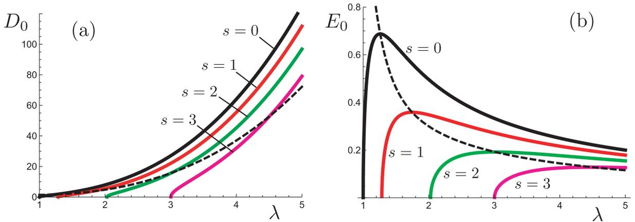
**Fig. 1.** Plots of (a)  $D_0$  versus  $\lambda$  and (b)  $E_0$  versus  $\lambda$  based on Eq. (31)<sub>1</sub> and the connection  $E_0 = \lambda^{-4}D_0$  for the neo-Hookean dielectric in equi-biaxial deformation, for values of non-dimensional pre-stress  $s = 0, 1, 2, 3$  (continuous curves). In (a) we also display the (dashed) curve of  $D_0 = \sqrt{(\lambda^6 + 5)}/3$ , the intersections of which with the continuous curves correspond to the maxima in (b).
