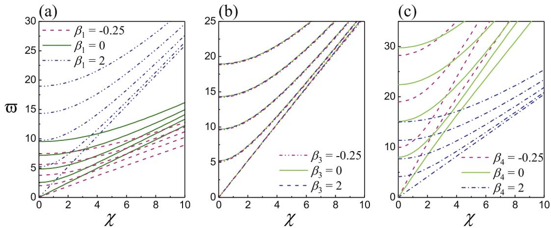
Fig. 11. Frequency spectra of the first five modes of the T waves in a functionally graded SEA tube with  $\lambda_z = 2.0$  and  $V^* = 0.4$ : (a) for various elastic moduli gradients  $\beta_1 = \beta_2$  (with  $\beta_3 = -0.25$  and  $\beta_4 = 1.0$ ); (b) for various permittivity gradients  $\beta_3$  (with  $\beta_1 = \beta_2 = 2.0$  and  $\beta_4 = 1.0$ ); (c) for various density gradients  $\beta_4$  (with  $\beta_1 = \beta_2 = 2.0$  and  $\beta_3 = 0$ ).
