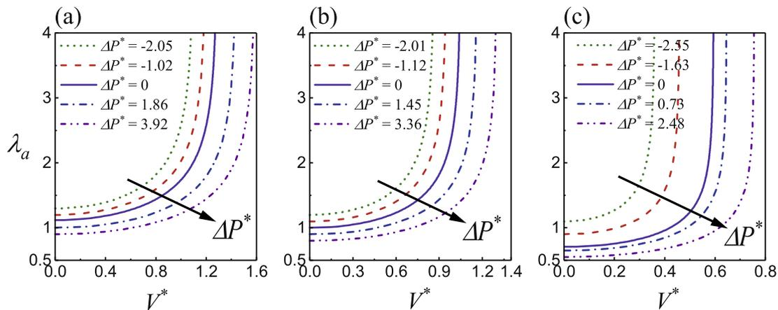
Fig. 4. Variations of the inner surface circumferential ratio  $\lambda_a$  with the dimensionless voltage  $V^*$  in a functionally graded SEA tube with material gradient  $\beta = \beta_1 = \beta_2 = \beta_3 = 5.0$ , for different values of pressure difference  $\Delta P^*$  and various axial pre-stretches  $\lambda_z$ : (a)  $\lambda_z = 0.8$ ; (b)  $\lambda_z = 1.0$ ; (c)  $\lambda_z = 2.0$ .
