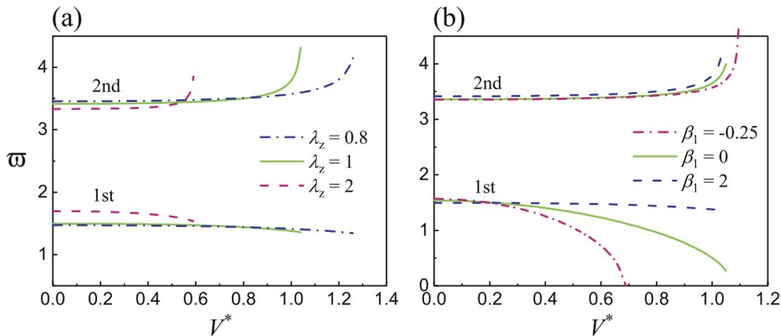
Fig. 15. The first two nonzero cut-off frequencies at  $\chi = 0$  of the L waves versus  $V^*$ : (a) for different axial pre-stretches  $\lambda_z$  (with  $\beta_i = 2.0$ ,  $i = 1, \dots, 4$ ); (b) for different material gradients  $\beta = \beta_i$  ( $i = 1, \dots, 4$ ) (with  $\lambda_z = 1.0$ ).
