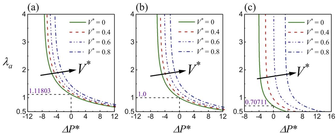
Fig. 3. Variations of the inner surface circumferential ratio  $\lambda_a$  with the dimensionless pressure difference  $\Delta P^*$  in a functionally graded SEA tube with material gradient  $\beta = \beta_1 = \beta_2 = \beta_3 = 5.0$ , for different values of voltage  $V^*$  and various axial pre-stretches  $\lambda_z$ : (a)  $\lambda_z = 0.8$ ; (b)  $\lambda_z = 1.0$ ; (c)  $\lambda_z = 2.0$ .
