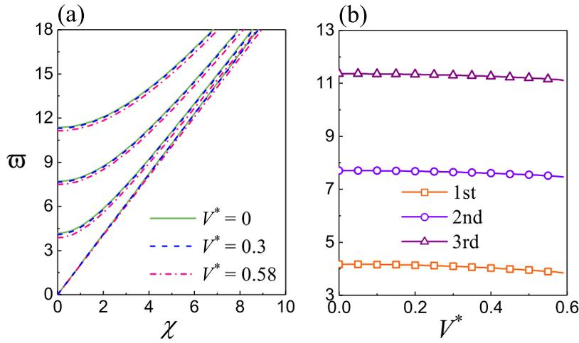
Fig. 10. (a) Frequency spectra of the first four modes of the T waves for different values of  $V^*$ , and (b) the first three nonzero cut-off frequencies at  $\chi = 0$  versus  $V^*$  in a functionally graded SEA tube with  $\beta_i = 2.0$  ( $i = 1, \dots, 4$ ) and  $\lambda_z = 2.0$ .
