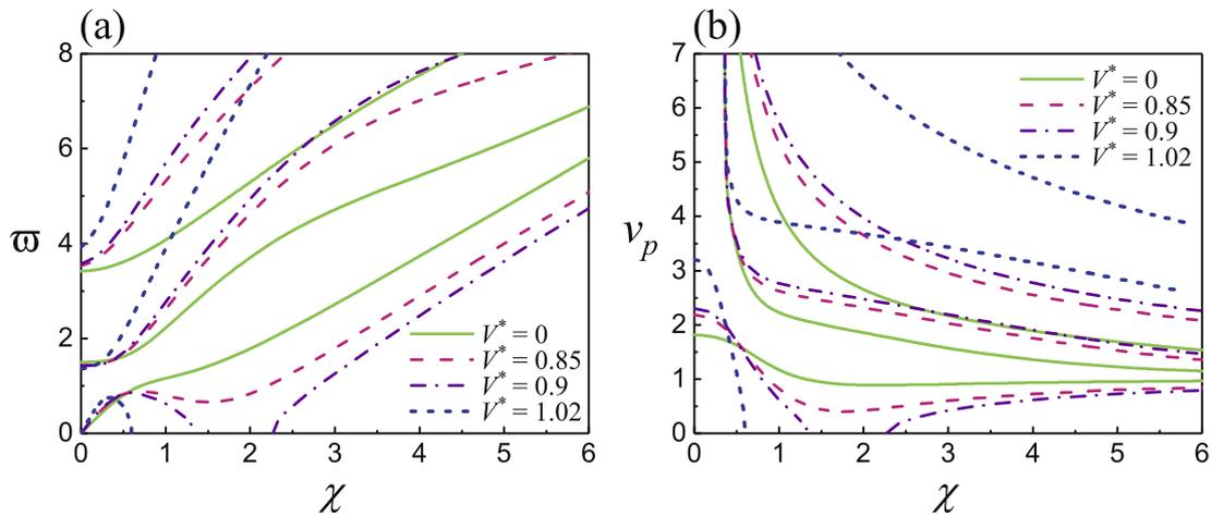
Fig. 14. Frequency spectra (a) and phase velocity spectra (b) of the first three modes of the L waves in a functionally graded SEA tube with  $\beta_i = 2.0$  ( $i = 1, \dots, 4$ ) and  $\lambda_z = 1.0$ , for different values of  $V^*$ .
