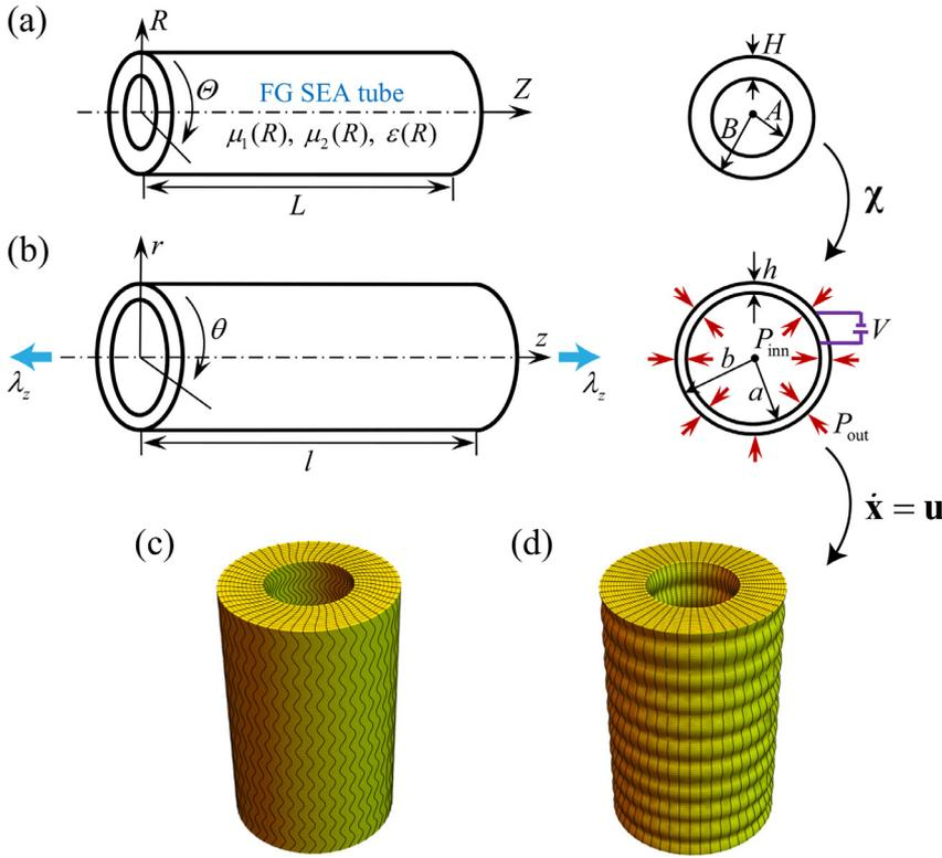
**Fig. 1.** Schematic diagram of a functionally graded SEA tube with its cylindrical coordinates and cross sections: (a) undeformed configuration before activation; (b) deformed configuration after activation induced by a combined action of axial pre-stretch  $\lambda_z$ , radial electric voltage  $V$  as well as internal ( $P_{inn}$ ) and external ( $P_{out}$ ) pressures. Incremental motion fields created by (c) torsional T-waves and (d) longitudinal L-waves.
