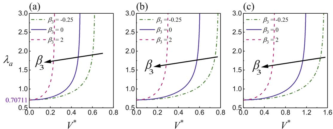
Fig. 5. Variations of the inner surface circumferential ratio  $\lambda_a$  with the dimensionless voltage  $V^*$  in a functionally graded SEA tube with  $\lambda_z = 2.0$  and  $\Delta P^* = 0$ , for different permittivity gradients  $\beta_3$  and three sets of elastic moduli gradients: (a)  $\beta_1 = \beta_2 = -0.25$ ; (b)  $\beta_1 = \beta_2 = 0$ ; (c)  $\beta_1 = \beta_2 = 2.0$ .
