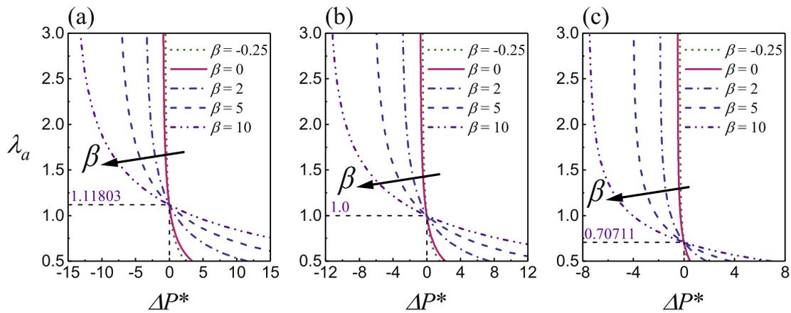
Fig. 2. Variations of the inner surface circumferential ratio  $\lambda_a$  with the dimensionless pressure difference  $\Delta P^*$  in a functionally graded SEA tube with no voltage  $V^* = 0$ , for different values of material gradient  $\beta = \beta_1 = \beta_2 = \beta_3$  and various axial pre-stretches  $\lambda_z$ : (a)  $\lambda_z = 0.8$ ; (b)  $\lambda_z = 1.0$ ; (c)  $\lambda_z = 2.0$ .
