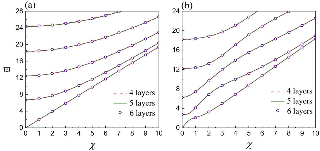
**Fig. 9.** Convergence analysis of frequency spectra of the first five wave modes obtained by the SSM for a functionally graded SEA tube with  $\beta_1 = \beta_2 = 5.0$ ,  $\beta_3 = \beta_4 = 1.0$ ,  $\lambda_z = 1.0$  and  $V^* = 0.2$ : (a) T waves; (b) L waves. Here  $n = 4, 5, 6$  is the number of the discretized thin layers.
