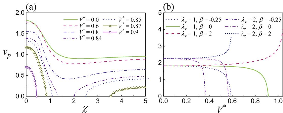
**Fig. 16.** (a) Phase velocity spectra of the lowest L wave mode in a homogeneous ( $\beta_i = 0, i = 1, \dots, 4$ ) SEA tube with  $\lambda_z = 1.0$  for different values of  $V^*$ . (b) Variations of the lowest L wave phase velocity at  $\chi = 0$  with  $V^*$  for different combinations of the axial pre-stretch  $\lambda_z$  and material gradient  $\beta = \beta_i$  ( $i = 1, \dots, 4$ ).
