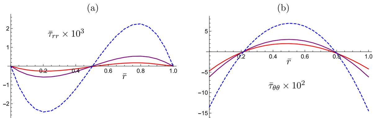
**Fig. 5.** Plots of (a) the radial stress  $\tau_{rr}$  and (b) the circumferential stress  $\tau_{\theta\theta}$  in scaled dimensionless form versus the normalized radius  $\bar{r}$  for the dimensionless voltage  $\bar{V} = 0.25$  and the following values of  $(\alpha_\varepsilon, \alpha_\mu)$ : red (0.4, 0.2); purple (0.4, 0.4); blue dashed (0.4, 0.6). (For interpretation of the references to color in this figure legend, the reader is referred to the web version of this article.)
