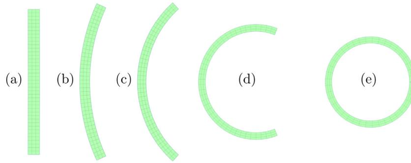
**Fig. 11.** (a) Undeformed rectangular plate cross section with aspect ratio  $L/A = 10$  and parameters  $\alpha_\varepsilon = -0.3, \alpha_\mu = -0.3$  and the following values of  $\bar{V}$ : (b) 0.3; (c) 0.4; (d) 0.5; (e) 0.5353.
