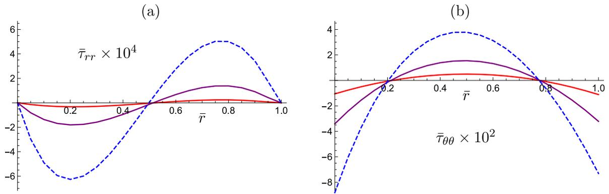
**Fig. 3.** Plots of (a) the radial stress  $\tau_{rr}$  and (b) the circumferential stress  $\tau_{\theta\theta}$  in scaled dimensionless form versus the normalized radius  $\bar{r}$  for the dimensionless voltage  $\bar{V} = 0.2$  and the following values of  $(\alpha_\varepsilon, \alpha_\mu)$ : red (0.1, 0.3); purple (0.4, 0.3); blue dashed (0.7, 0.3). (For interpretation of the references to color in this figure legend, the reader is referred to the web version of this article.)
