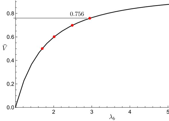
**Fig. 10.** Plot of  $\bar{V}$  versus  $\lambda_b$  for the parameters  $\alpha_\varepsilon = -0.3, \alpha_\mu = 0.3$  and aspect ratio  $L/A = 10$ . The red bullet points are associated with the values 0.5, 0.6, 0.7, 0.756 of  $\bar{V}$  in Fig. 9(b)–(e), respectively.
