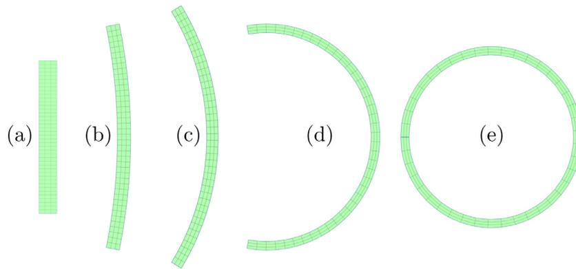
**Fig. 7.** (a) Undeformed rectangular plate cross section with aspect ratio  $L/A = 10$  and  $\bar{V} = 0.3$ , with parameters  $(\alpha_\varepsilon, \alpha_\mu)$ : (b)  $(-0.3, 0.3)$ ; (c)  $(-0.45, 0.3)$ ; (d)  $(-0.6, 0.3)$ ; (e)  $(-0.6511, 0.3)$ .
