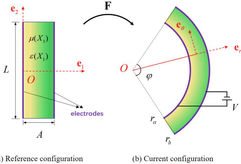
**Fig. 1.** A block of FGDE with continuously varying shear modulus  $\mu(X_1)$  and permittivity  $\varepsilon(X_1)$  through the thickness, coated with two compliant electrodes. The layer bends when loaded with a voltage  $V$  across the electrodes, with the bending angle  $\varphi$ .
