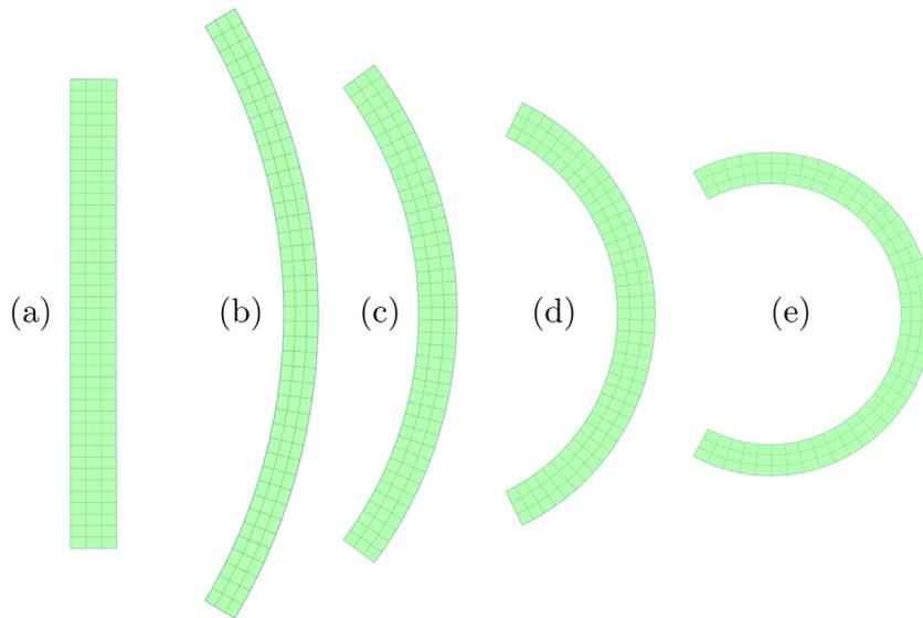
**Fig. 4.** (a) Undeformed rectangular plate cross section with aspect ratio  $L/A = 10$ . (b)–(d) plate bent by application of a dimensionless voltage  $\bar{V} = 0.25$  with the following values of  $(\alpha_\varepsilon, \alpha_\mu)$ : (b) (0.4, 0.2); (c) (0.4, 0.4); (d) (0.4, 0.6), and (e) with  $\bar{V} = 0.4$  and  $\alpha_\varepsilon = 0.4, \alpha_\mu = 0.4$ .
