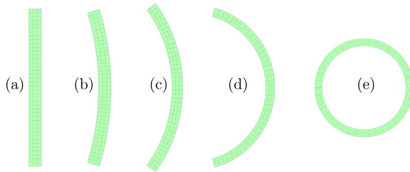
**Fig. 2.** (a) Undeformed rectangular plate cross section with aspect ratio  $L/A = 10$ . (b)–(e) plate bent by application of a dimensionless voltage  $\bar{V} = 0.2$  with the following values of  $(\alpha_\varepsilon, \alpha_\mu)$ : (b) (0.3, 0.3); (c) (0.7, 0.3); (d) (1.1, 0.3); (e) (1.521, 0.3).
