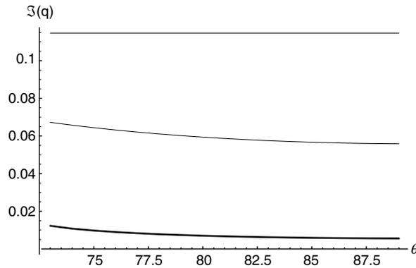
Fig. 5. Attenuation factors for Rayleigh (thin curves) and Stoneley (thick curve) wave speeds for a bi-material made of Douglas pine ( $Y$ -cut) and of carbon/epoxy (rotated  $Y$ -cut about the  $Z$ -axis), in the range of common existence.
