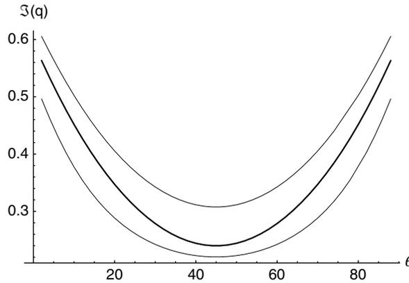
Fig. 3. Attenuation factors for Rayleigh (thin curves) and Stoneley (thick curve) wave speeds for a bi-material made of aluminum (rotated Y-cut about the Z-axis) and of tungsten (symmetrically rotated Y-cut about the Z-axis).
