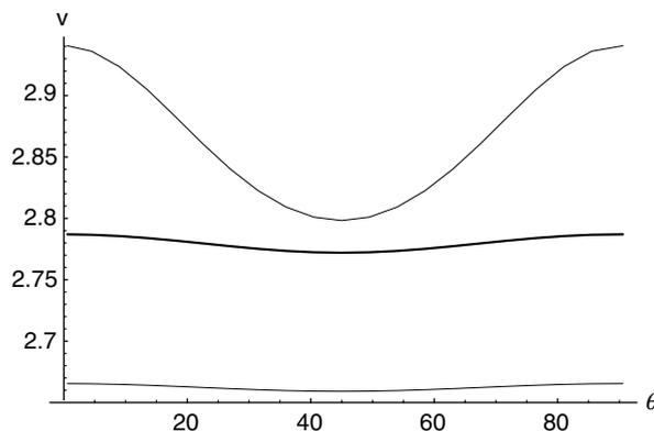
Fig. 2. Rayleigh (thin curves) and Stoneley (thick curve) wave speeds for a bi-material made of aluminum (rotated Y-cut about the Z-axis) and of tungsten (symmetrically rotated Y-cut about the Z-axis).
