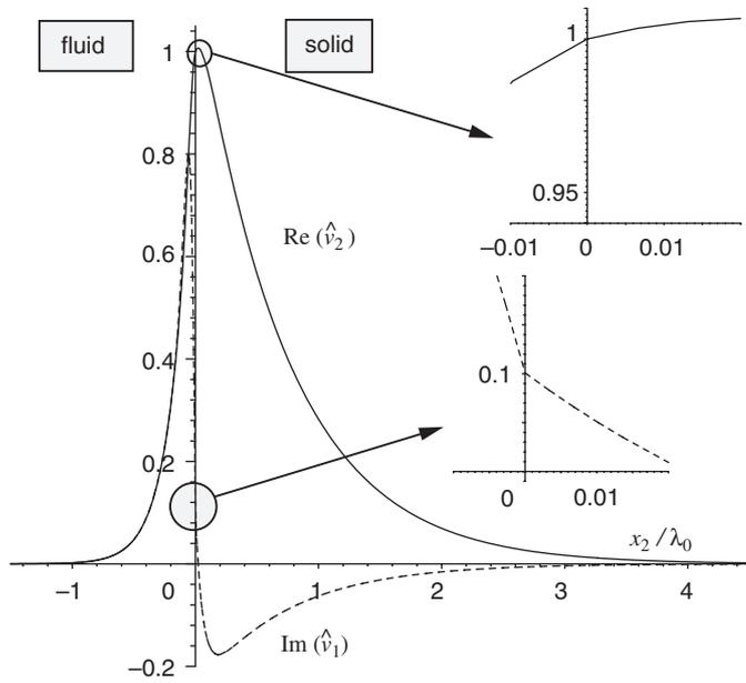
Fig. 1. Depth profiles as functions of  $x_2/\lambda_0$  of the velocity components of the acoustic wave:  $x_2$  (normal) component—continuous curve;  $x_1$  (tangential) component—dotted curve. The zooms show continuity of these components and discontinuity of their derivatives.
