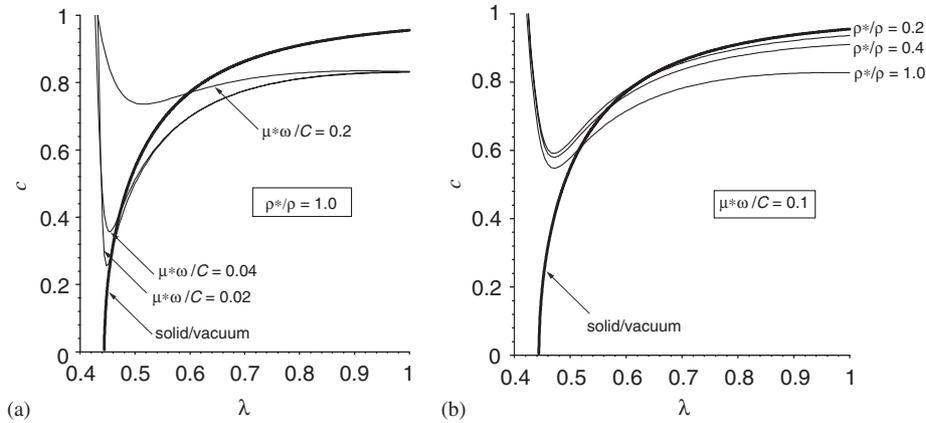
Fig. 2. Normalized wave speed for a neo-Hookean solid under normal equi-biaxial pre-strain and a viscous fluid: (a)  $\rho^*/\rho = 1.0$  and  $\mu^*\omega/C = 0.02, 0.04, 0.2$ ; (b)  $\rho^*/\rho = 0.2, 0.4, 1.0$  and  $\mu^*\omega/C = 0.1$ . The thick curves are for an unloaded solid half-space.
