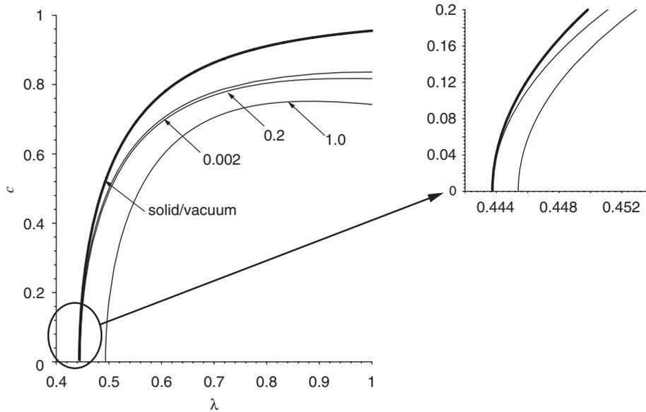
Fig. 3. Normalized wave speed for a neo-Hookean solid under normal equi-biaxial pre-strain and a viscous fluid with  $\rho^*/\rho=1.0$  and  $\mu^*k/\sqrt{\rho C}=0.002, 0.2, 1.0$  (indicated by the arrows) for the compressive range  $0.4 < \lambda < 1$ . The zoom shows the details for  $\mu^*k/\sqrt{\rho C} = 0.002, 0.2$  for  $0.442 < \lambda < 0.445$  range. The thick curve corresponds to the solid half-space with no fluid loading.
