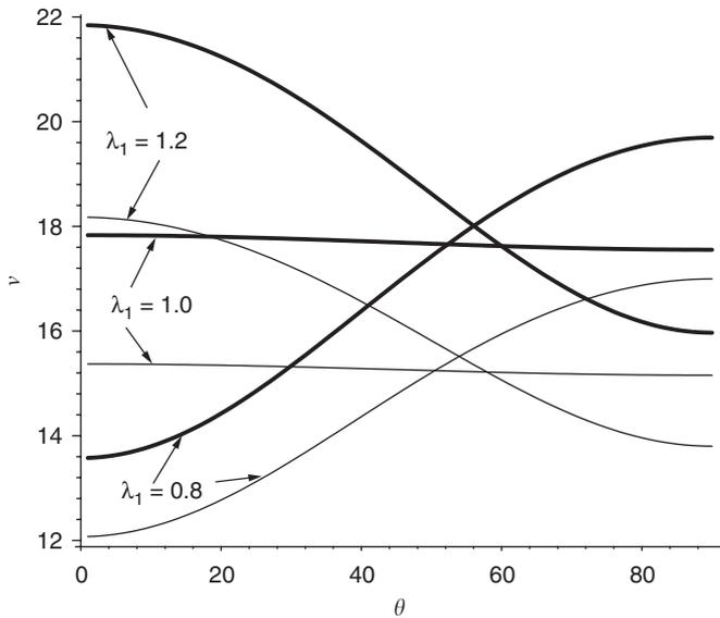
Fig. 4. Influence of propagation angle  $\theta$  on the speed  $v$  of a wave at the interface between a viscous fluid and a deformed neo-Hookean solid (thin curves). The thick curves represent the wave speed in the absence of fluid loading.
