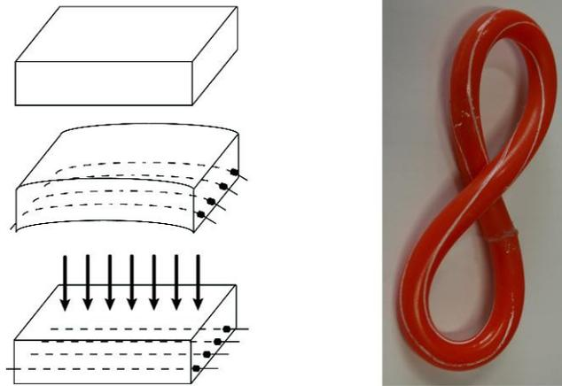
FIG. 1. On the left: Stabilizing a bridge span made of concrete by reinforcing it with steel rods put under tension. Once the span is put in place and subject to loads, the concrete is compressed everywhere. On the right: Destabilizing a ring by twisting a polyurethane rod before gluing its two ends together. For a large enough pretwist, the ring folds unto itself in an eight-shape.
