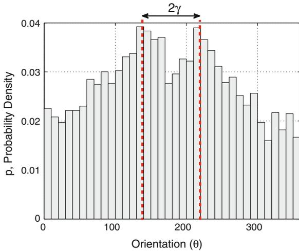
**FIGURE 2.** Histogram of collagen orientations. The two distinct peaks correspond to the preferred orientation of the two fiber families. The angle,  $\gamma$ , is half the distance between the two peaks i.e.  $\gamma = 41^\circ$ .
