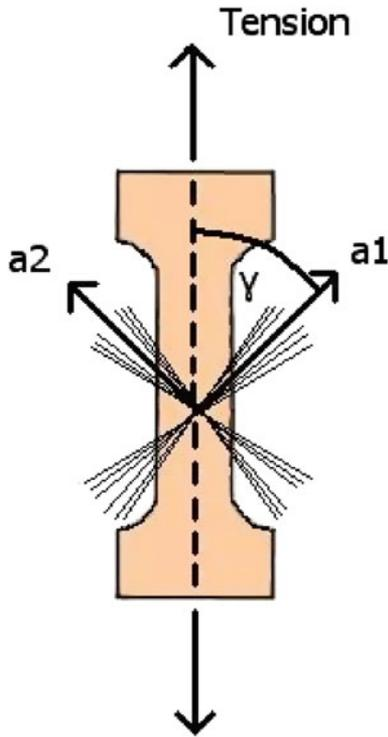
**FIGURE 3.** Lattice structure of crossing collagen fibres with fibre dispersion taken into account.
