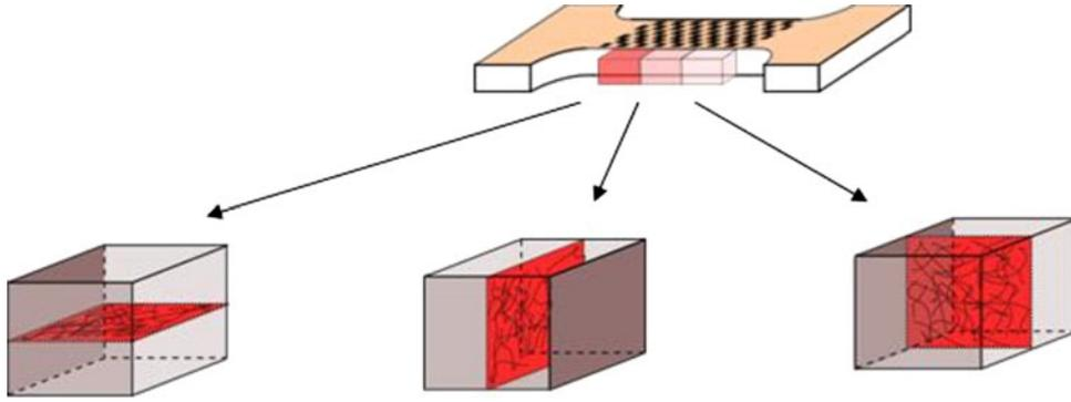
**FIGURE 4.** Biopsies of skin samples for purpose of histological staining. Note that the biopsies have been sliced in three orthogonal planes.
