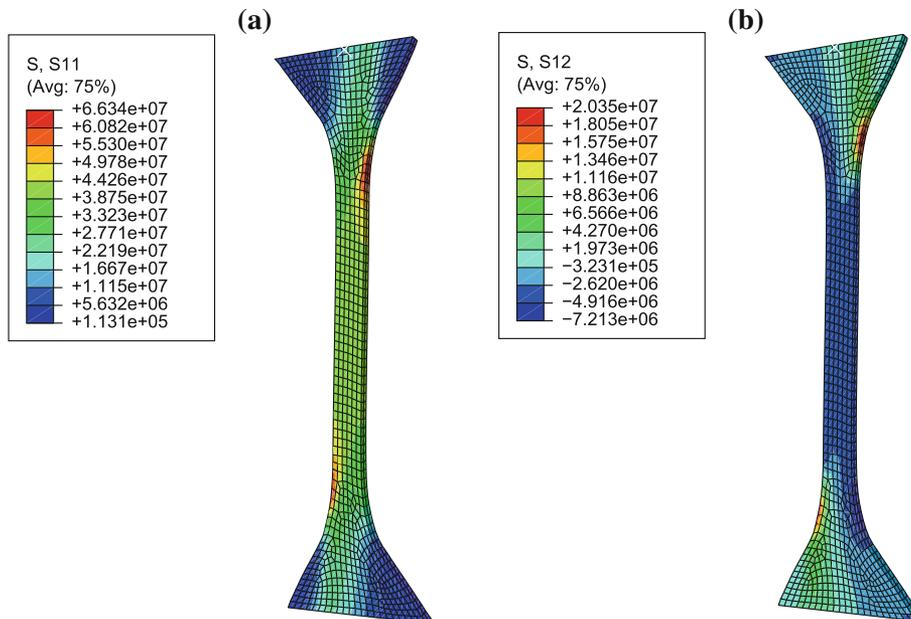
**FIGURE 12. Cauchy stress in Pa of a non-symmetric sample strained by 30% (a)  $\sigma_{11}$  (b)  $\sigma_{12}$ .**
