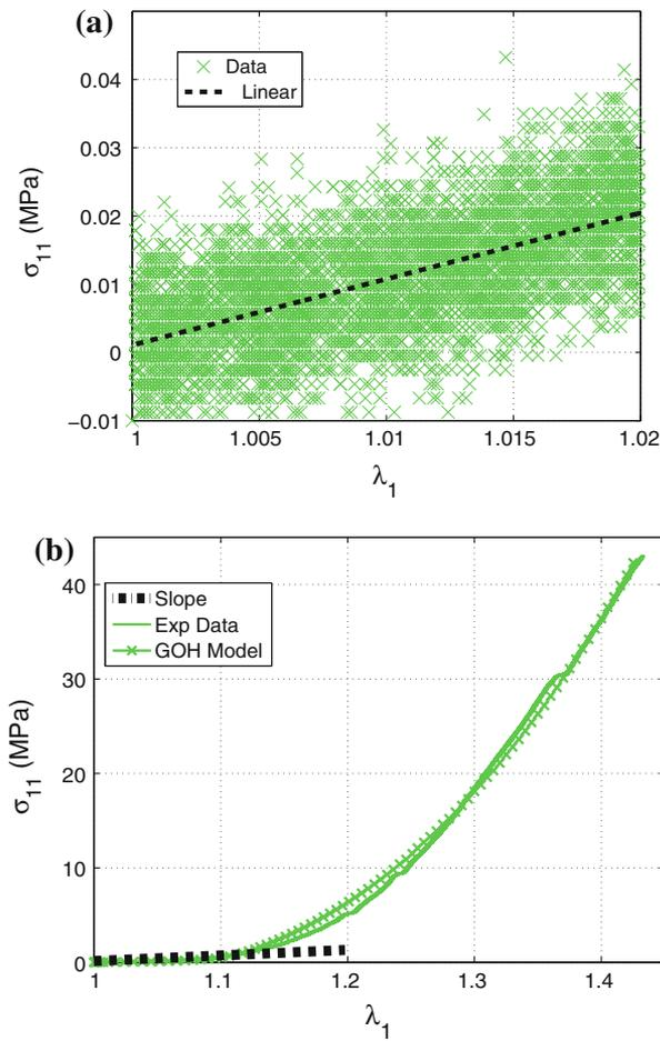
**FIGURE 9.** Nonlinear curve fitting to obtain the constitutive parameters:  $\mu$  and  $k_1$  are related to the early (infinitesimal) stress-strain part of the graph, see (a);  $k_2$ , to the rest of the curve.
