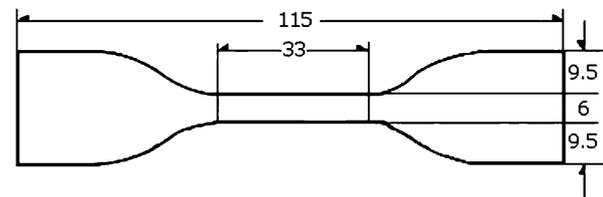
**FIGURE 7.** Dimensions of test specimen (mm).
