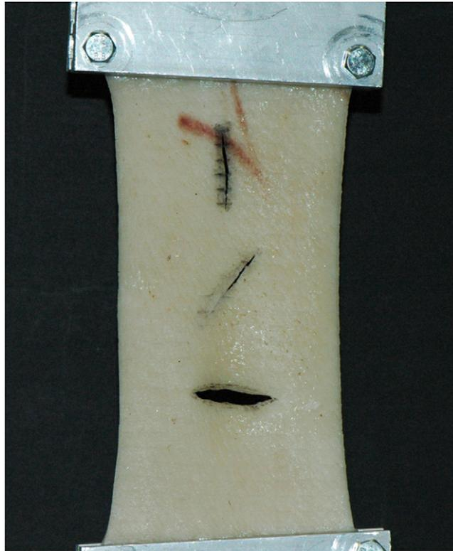
**Fig. 1.** Cutting through pig skin: a clamped sample of pig skin is put under tension, after 3 cuts have been performed, parallel (top), oblique (center) and perpendicular (bottom) to the tensile force.
