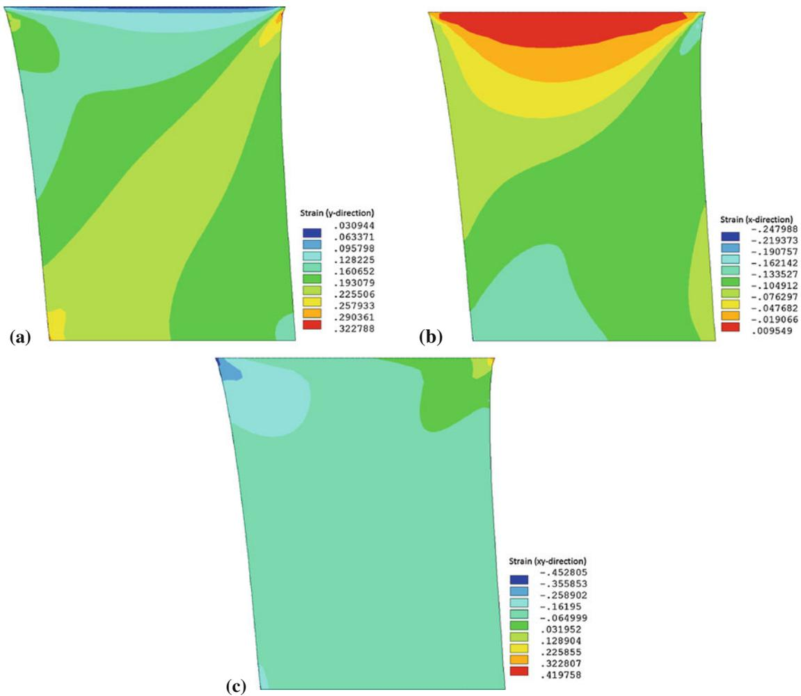
**Fig. 4** Contour plots of **a** normal strain; **b** transverse strain; **c** shear strain
