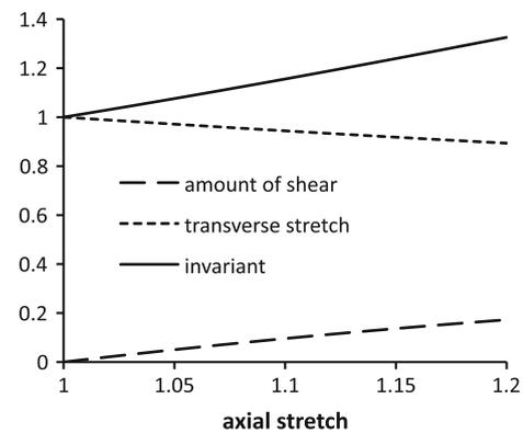
Fig. 5 Typical transverse stretch, shear and  $I_4$  results
