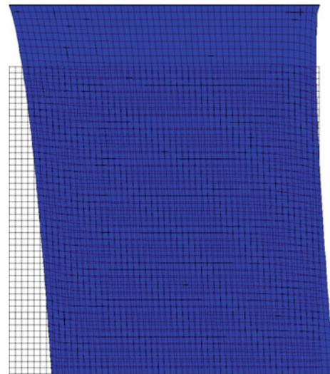
**Fig. 9** Initial and final configurations with  $\lambda_2 = 1.2$  for 80° initial fibre orientation
