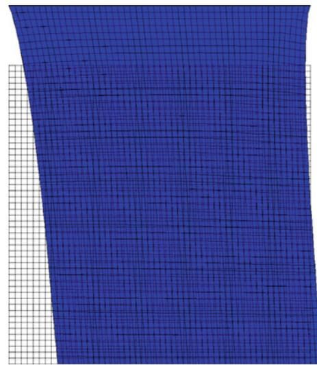
**Fig. 3** Initial configuration and final configuration with  $\lambda_2 = 1.2$  for  $45^\circ$  initial fibre orientation
