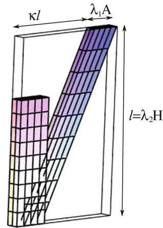
**Fig. 1** A cuboid of hyperelastic material reinforced with one family of parallel fibers can deform homogeneously when subjected to a tensile force only, as a combination of triaxial stretch (with stretch ratios  $\lambda_i$ ) and simple shear (with amount of shear  $\kappa$ )
