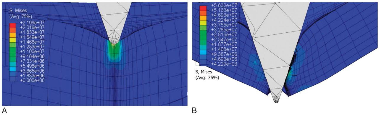
**FIGURE 2.** Numerical progression of a carving knife through human skin (units in Pa). A, indentation prior to initial penetration; B, full perforation.
