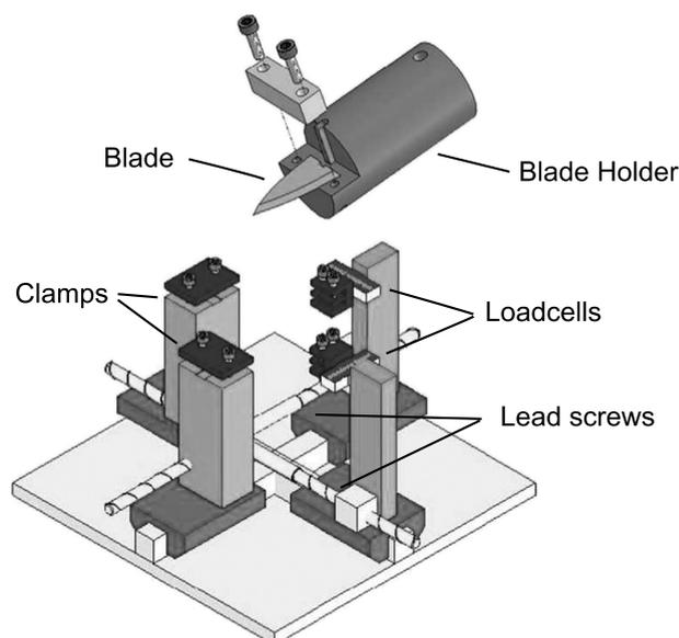
FIGURE 1. Illustration of blade holder and biaxial device.<sup>10</sup>
