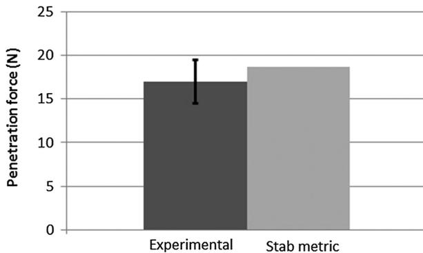
**FIGURE 5.** Comparison of experimental data for carving knife penetrating human skin at quasi-static speeds to the same stab-metric prediction.
