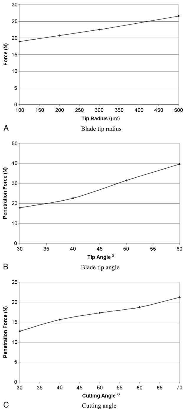
FIGURE 4. The maximum penetration force as a function of the characteristic blade dimensions.
