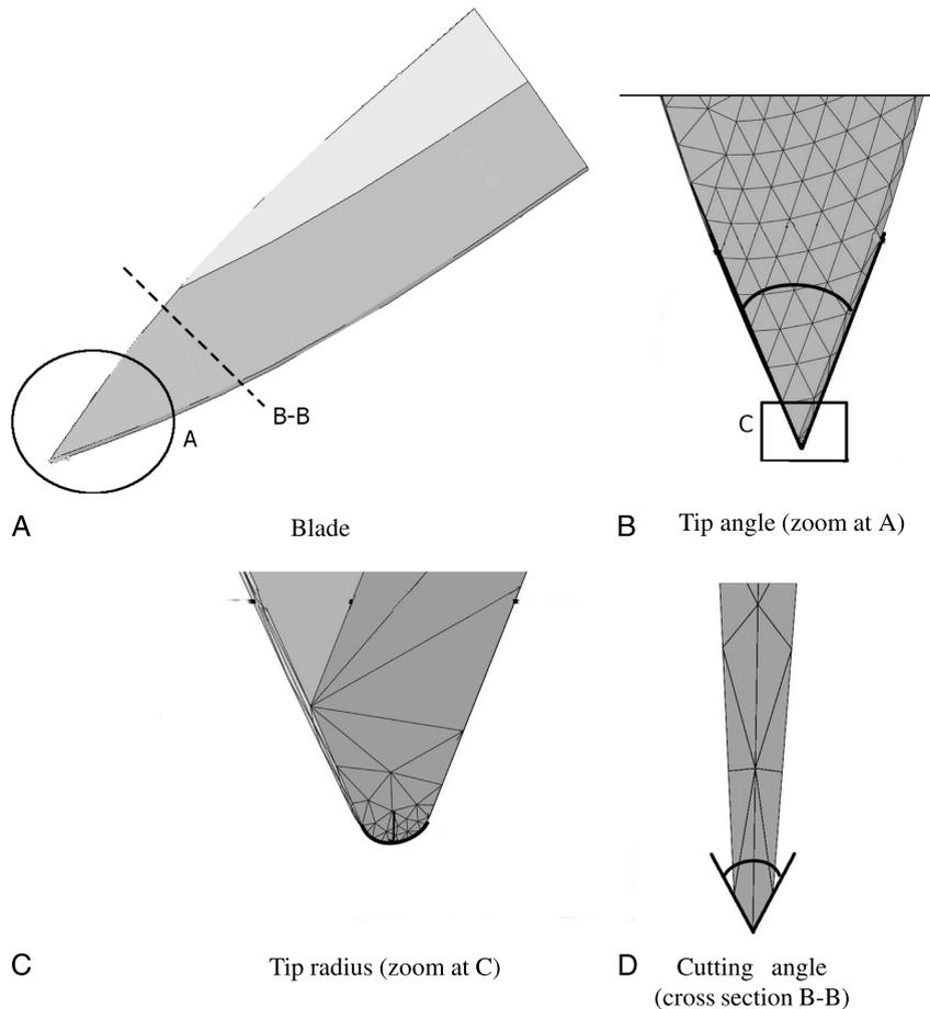
**FIGURE 3.** Indicative blade dimensions (A) blade, (B) tip angle (zoom at A), (C) tip radius (zoom at C), (D) cutting angle (cross section B-B).
