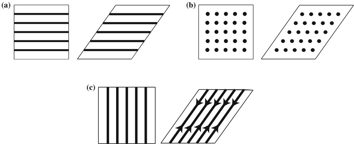
**Fig. 1** Schematics of **a** longitudinal shear, **b** transverse shear and **c** perpendicular shear. In **a** and **c**, the *dark lines* represent the fibres. In **b**, the *darkened circles* denote fibres out of the plane of the page. The *arrows* in **c** indicate the resistive forces developing in the stretched fibres in response to the simple shear: this shear mode provides a simple mechanism to model negative Poynting effects
