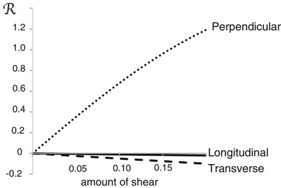
**Fig. 3** Plots of  $\mathcal{R}$  (relative magnitude of normal stress with respect to applied shear stress) for different shearing modes of one model of a solid reinforced with one family of fibres
