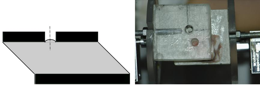
**Fig. 4.** Poynting effect for the large ( $K=1$ , angle= $45^\circ$ ) simple shear of porcine brain matter ( $19 \times 19 \times 3$  mm): without the platens, the sample would expand in the 2-direction. This tendency is revealed by drilling a hole in one platen and observing from above the drilled platen that the exposed area bulges outwards (it is clearly visible to the naked eye, but difficult to capture in the photograph).
