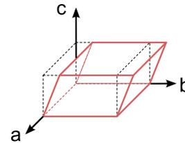
**Fig. 2.** Simple shear deformation. Dotted lines: sample in the undeformed configuration; solid lines: deformed sample.
