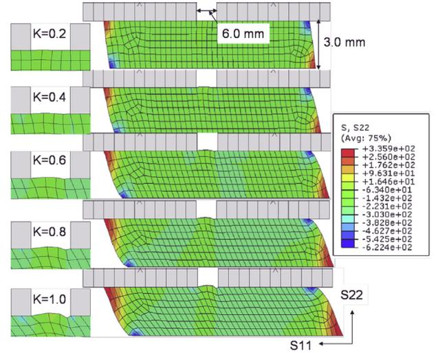
**Fig. 5.** Finite Element simulation of simple shear experiment conducted in Fig. 4. The scale on the right indicates the normal stress magnitude  $S_{22}=\sigma_{22}$  at  $K=1$ . The simulation confirms that outside localized edge areas, the stress distribution is largely homogeneous throughout the sample, and that the Poynting effect will make the material bulge out in the absence of a normal compressive force.
