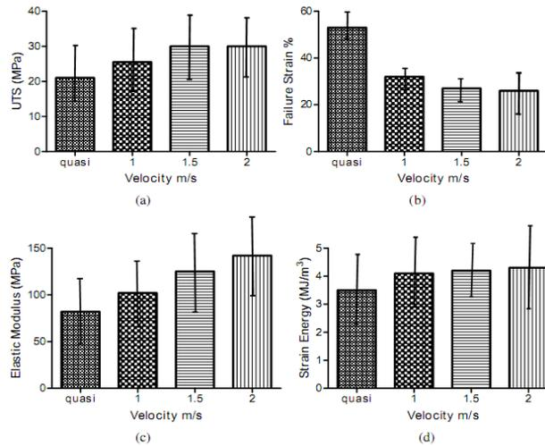
Fig. 1: Means and standard deviations at different test speeds; quasi-static (N=55), 1m/s (N=18), 1.5 m/s (N=11), 2m/s (N=4).
