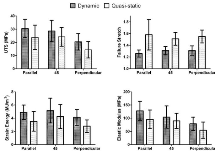
Fig. 2: Effect of sample orientation at dynamic strain rates (N=33, 14.5-29 s<sup>-1</sup>) and at quasi static strain rates (N=55, 0.83 s<sup>-1</sup>).
