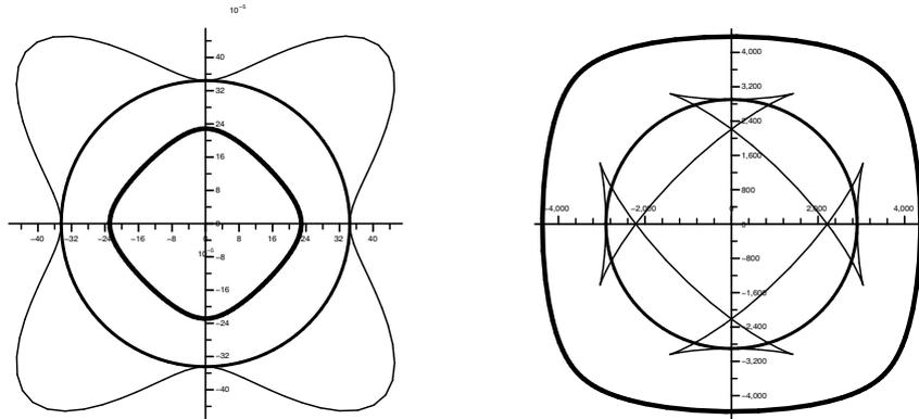
Figure 3: Homogeneous bulk waves in a plane of symmetry for copper (cubic symmetry). On the left: slowness surface (s/m); On the right: wavefronts, represented by the group velocity (m/s). Values used:  $d_{11} = 17.0$ ,  $d_{12} = 12.0$ ,  $d_{44} = 7.5$  ( $10^{10}$  Pa), and  $\rho = 8.9 \times 10^3$  ( $\text{kg/m}^3$ ).
