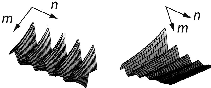
Figure 2: Inhomogeneous waves. On the left: the planes of constant phase are orthogonal to the planes of constant amplitude; On the right: they are at  $45^\circ$ .
