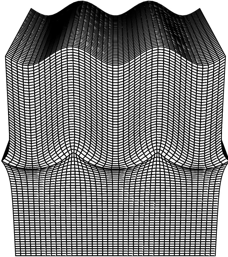
Figure 10: Displacements due to a Stoneley wave at the interface between Nickel (top) and Silica (bottom). Its amplitude decays exponentially with distance from the interface. The Stoneley wave speed (2921 m/s) is very close to the speed of the bulk shear wave in Nickel (2922 m/s), which is why the decay occurs over much greater distances in the upper half-space than in the bottom one.
