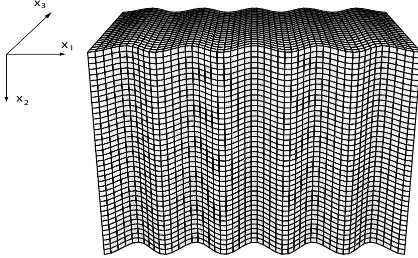
Figure 4: A shear horizontal surface wave in a homogeneous semi-infinite solid. It propagates in the  $x_1$ -direction, and is polarized in the  $x_3$ -direction. Its amplitude remains constant with the depth  $x_2$ . It is unlikely to be observed at all.
