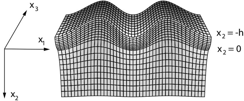
Figure 8: Displacements due to a Love surface wave in a superficial layer with shear modulus  $\hat{\mu}$  and mass density  $\hat{\rho}$ , rigidly bonded to a semi-infinite substrate with shear modulus  $\mu = 2\hat{\mu}$  and mass density  $\rho = \hat{\rho}$ . Here the wave propagates with a wavelength which is 4 times  $h$ , the layer thickness, and only the fundamental mode exists.
