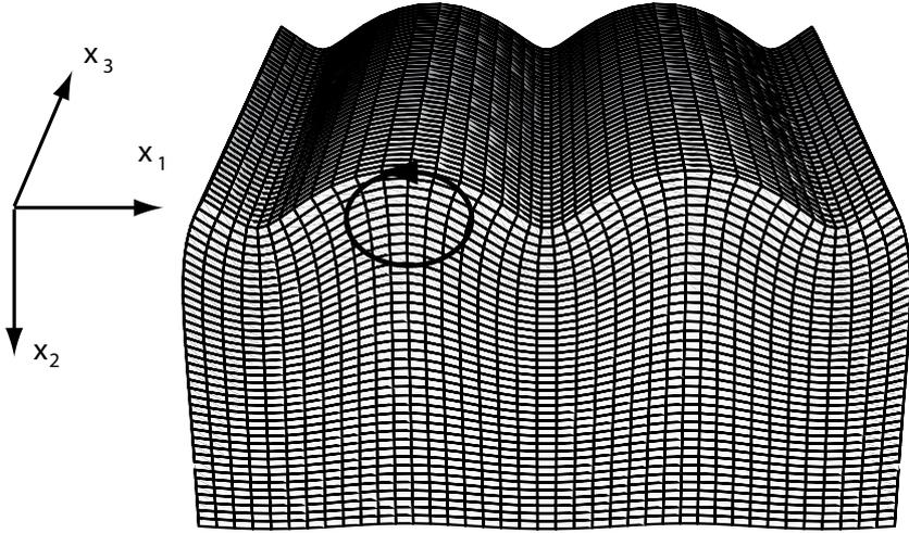
Figure 6: A Rayleigh surface wave in a homogeneous semi-infinite solid with Poisson ratio  $\nu = 1/4$ . Its amplitude decays exponentially with depth and is polarized in the sagittal plane (which includes the direction of propagation  $x_1$  and the normal to the boundary  $x_2$ ). The ellipse of polarization is described in a retrograde manner near the surface.
