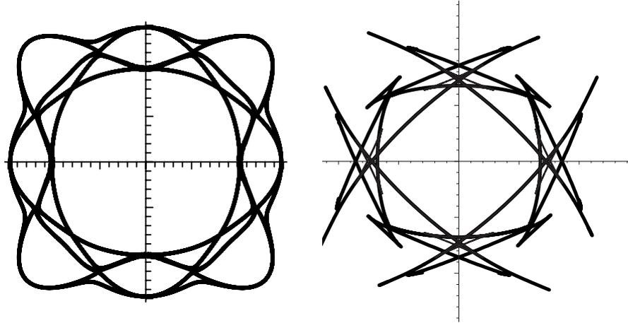
Figure 9: Surface waves in a plane of symmetry for Copper (cubic symmetry). On the left: slowness surface; On the right: wavefronts.
